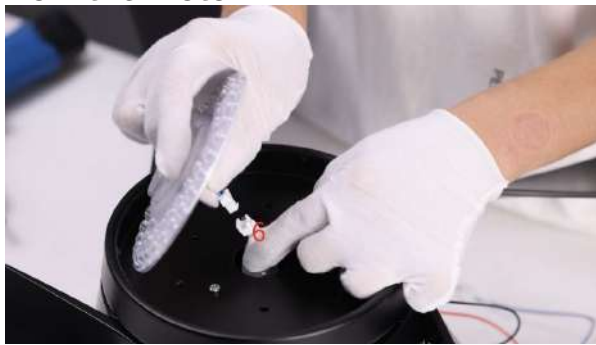
9. Connect the light source with the wires from the motor
