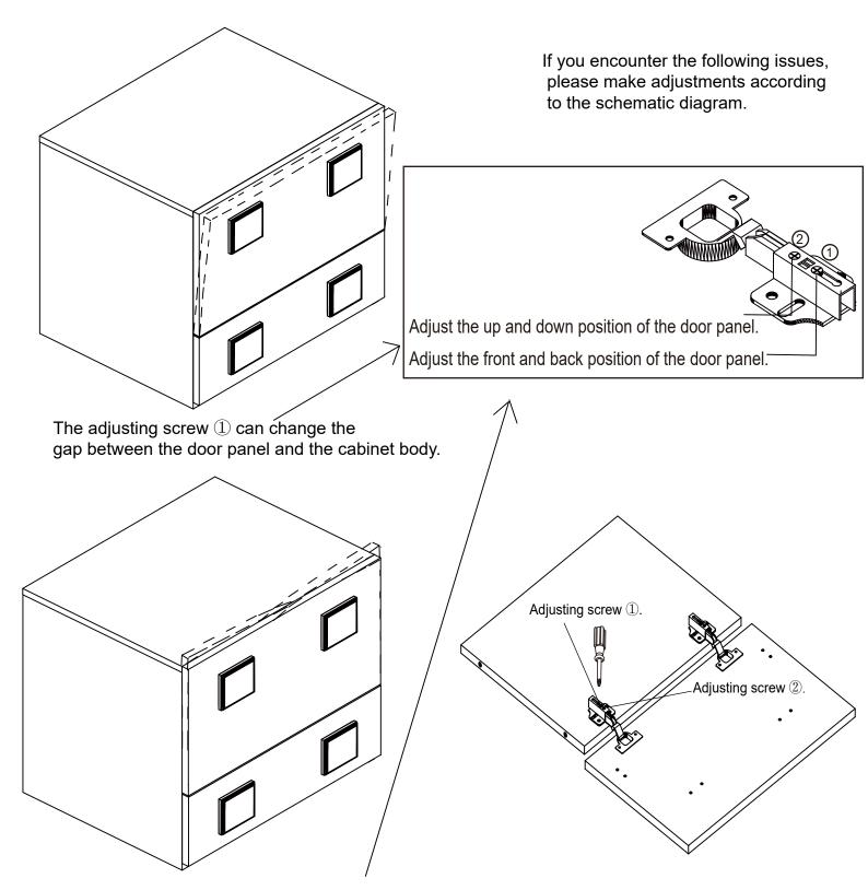
Adjusting screw ② can change the gap between the door panel and the cabinet body up and down.
