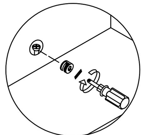
Use a screwdriver to lock in the direction of the "+" sign    Disassemble along the direction of "-" sign
