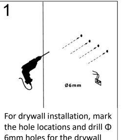
6mm holes for the drywall anchors. Install a junction box behind the mirror for power connections.
