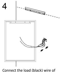
the Dimming driver cable (white) to wall switch if used. Connect the load (black) wire of the Touch Switch cable (black) to hot wire.
