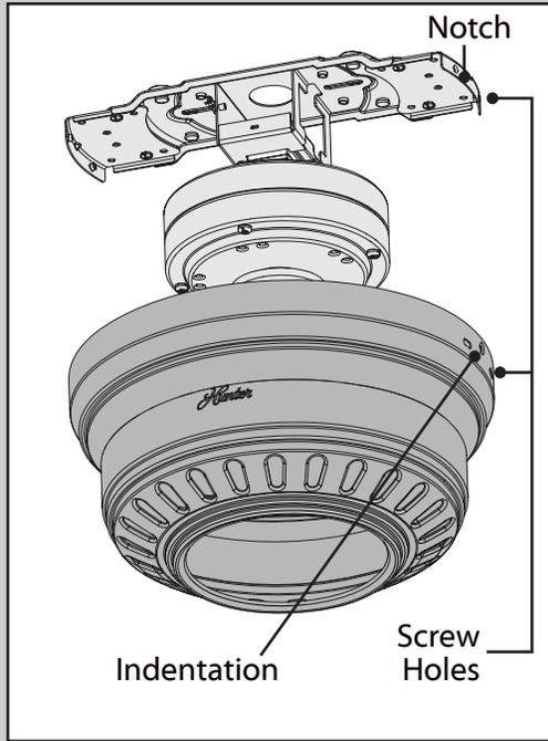
Raise the motor housing up over the motor and ceiling bracket. Turn the motor housing so the screw holes align and the indentation in the housing locks into place with the notch in the ceiling bracket. **The motor housing is not secured until the next step is complete. Do not leave unattended.**
