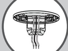
**Note:** To connect the wires, hold the bare metal leads together and place a wire connector over them, then twist clockwise until tight.
