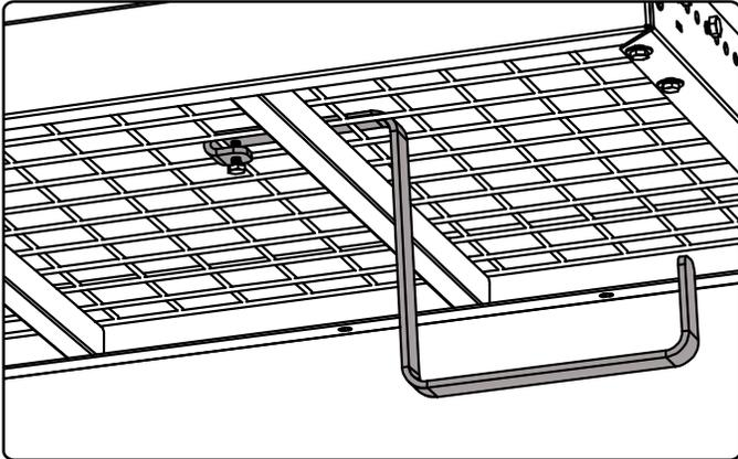
**1** From the **bottom** of the Pro Wall Mounted Shelf, determine location for utility hook to be installed; slide the folded end with bolt holes of the S-hook up through the opening in the wire grid.
