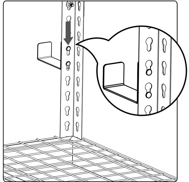
**Note:** When installing more than one J-Hook on the same side of the vertical angle post, start with the lowest position and install the next hook above.
