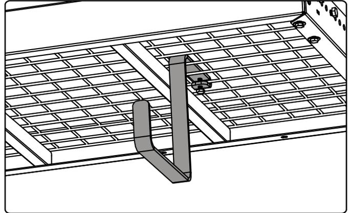
**2** Slide the folded end with bolt holes of the S-hook onto the wire grid.
