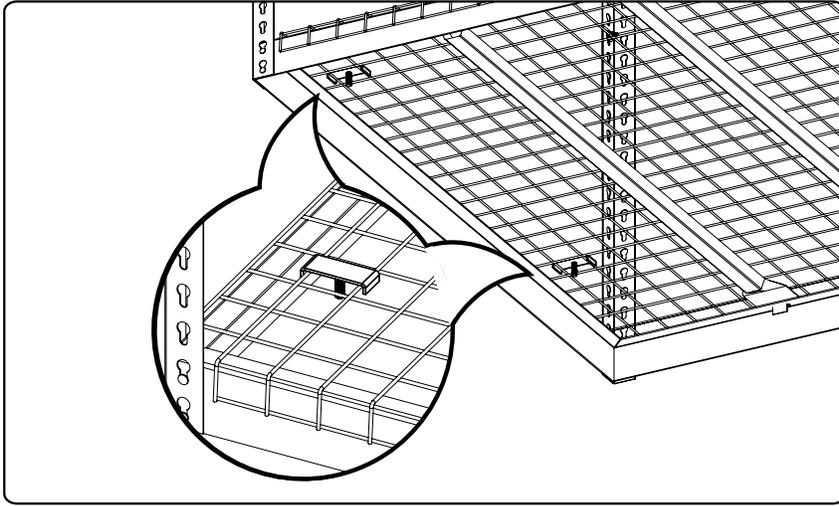
**Note:** Install grid clip on top layer of wires, not bottom wires.
