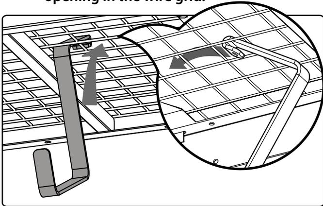
**3** Screw in the 5/16" dia x 1/2" bolt to secure the utility hook and tighten using a wrench.
