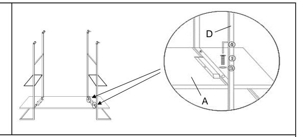
Attach Tray(A) to Right Side Panel(D) using Bolts(1) and Washers(3) with Allen Key(4) as pictured above.
