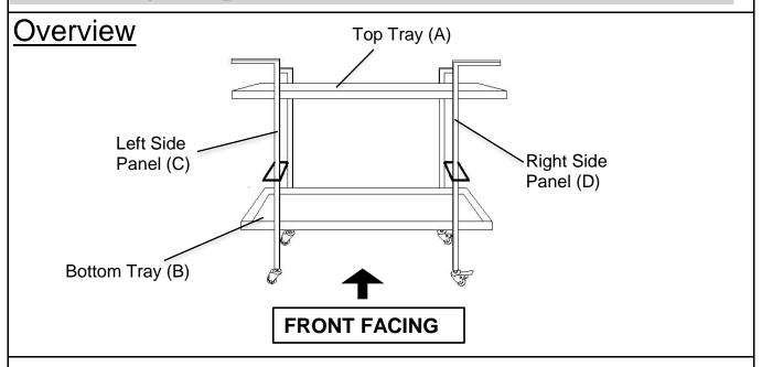
This Trolley has multiple parts and may require up to 30 minutes to assemble. To give you an overview of the Trolley parts, the above picture is to help you put the various parts into perspective. Please read through the instructions below to familiarise yourself with the parts and steps before assembly.
