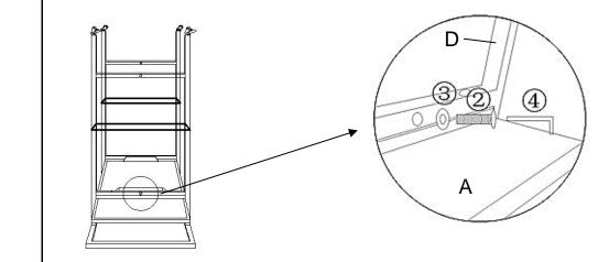
Attach Right Side Panel(D) to the Top Tray(A) through the pipe into the wooden block using Bolt(2) and Washer(3) with Allen Key(4).
