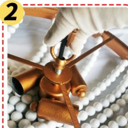
Pass wire go through lamp frame, then screw the loop for fixing the bulbs fixture body.
