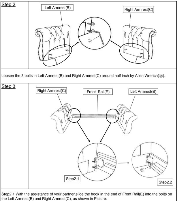
Step2.2 Tighten the Bolts by Allen Wrench(2).
