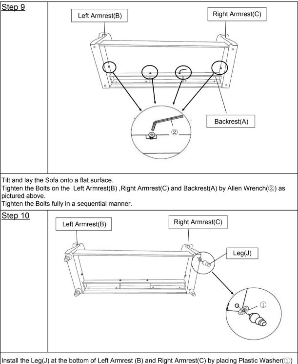
Install the Leg(J) at the bottom of Left Armrest (B) and Right Armrest(C) by placing Plastic Washer(1) on the threaded stem.
