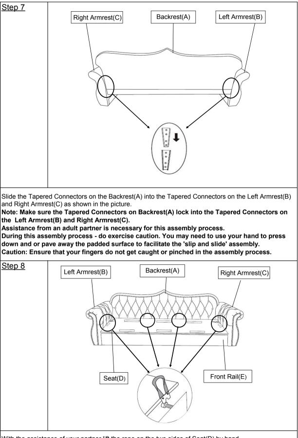
With the assistance of your partner, lift the rope on the two sides of Seat(D) by hand. Put the Seat(D) on the wood bar of the Front Rail(E) and then slowly place it down as shown above. **Note:All the u-shaped iron sheet need clamped to the bolt.**
