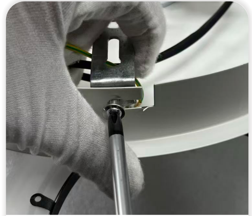
15 Lock the side screws of the base.
