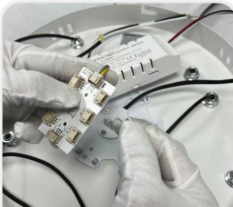
11 Insert the lamp holder wire into the terminal block.
