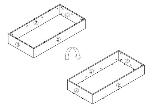
Connect the ② and ③ Panel with ① Panel. Then tighten all panels with B(3 in 1 locking) at holes position clockwise.As below shown:
