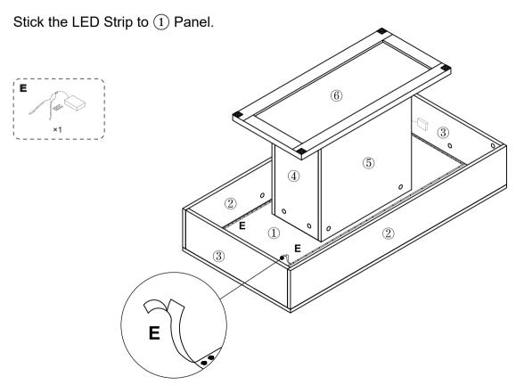
Before installation, please remove the adhesive protective film of the LED lamp belt, insert the buckle into the lamp belt, and follow the instructions to attach the lamp belt
