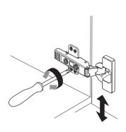
Screw C for door up & down adjustment.
