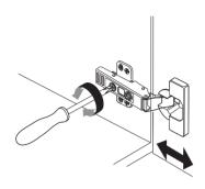
Screw A for door in & out adjustment.
