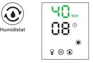
After reaching the preset humidity, the machine will stop humidifying. When the ambient humidity falls below the preset humidity, it will resume working again. After reaching 90%, press the Humidistat button again to exit constant humidity mode, and press it yet again to return to the initial humidity setting of 40%.
