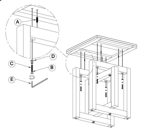
Carefully assemble the leg (2), frame stretcher (3) and locate the position on the top (1) make sure the position are all correctly place and insert the Dowel (A), Bolt (B), Lock Washer (C), Flat Washer (D)as shown, and tighten with the Allen Key (E) provided.
