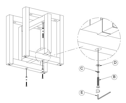
Assemble the leg (2) and frame stretcher (3) use Bolt (B), Lock Washer (C), Flat Washer (D)as shown, and tighten with the Allen Key (E) provided.
