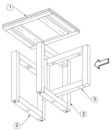
Place top panel (1) on the flat soft surface. Additional soft cloth layer may require to prevent unnecessary scratches or damages on the table top during installation. Insert the cross stretcher assembly (3) into the leg frame assembly (2) as shown.
