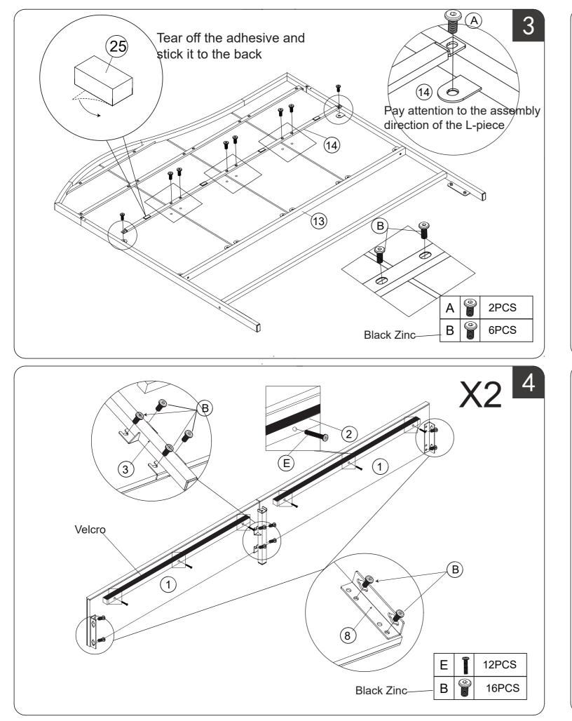
component 12 2. Screw all the parts sequentially, do not fully tighten all the screws until you complete all the installation. (C)0 UP (13) (A)B B В ₽(A Note: 1, Arrange part 21, 22, 23, 24 in the stainless steel
