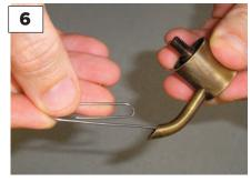
First insert the paper clip into the spout. Some force will be required to drive the clip through the entire length of the spout and fully clear the debris.
