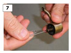
Next, insert the paper clip into the threaded neck. Again, force will be required to drive the clip through the entire length of the neck and clear the debris.
