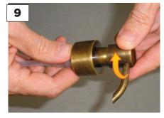
Screw the top portion back on the base: Hold the plastic tube firmly and turn the top portion clockwise. Reinstall the finished pump assembly on your dispenser.
