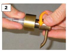
Hold the plastic tube containing the spring mechanism (as shown above) and unscrew the top portion by turning it counter-clockwise.
