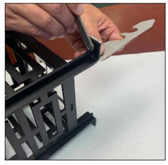
Use wrench provided to tighten locking screw.
