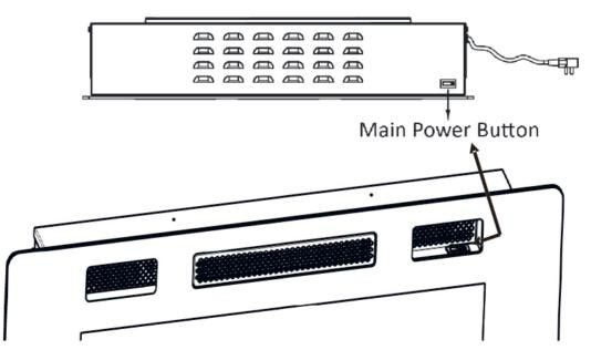
Note: Make sure the Main Power Switch is turned on before operating.
