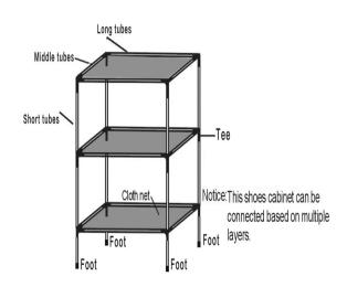
Taking out 4pcs plastic tee, 2pcs long rail tubes, 2pcs short rail tubes. Inserting plastic tee based on direction of arrows, then inserting small cloth to long rail tubes, lying flat, taking out 4pcs supporting tubes to insert plastic tee. According to pictures to connect:
