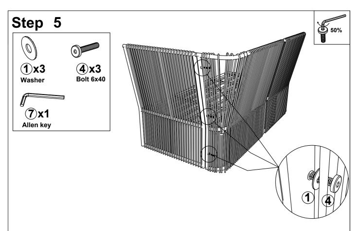
Tighten Bolt (4), Flat Washer (1) With Allen key (7)
