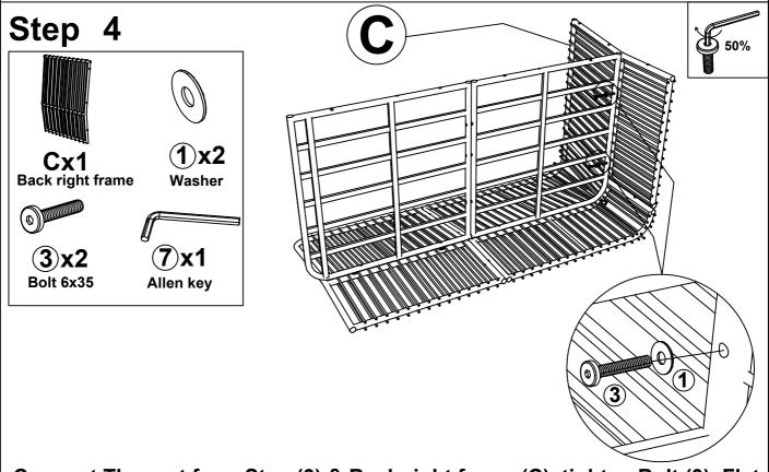
Connect The part from Step (3) & Back right frame (C), tighten Bolt (3), Flat Washer (1) With Allen key (7)
