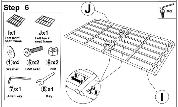
Connect The Left front seat frame (I) & Left back seat frame (J), tighten Bolt (5), Nut (6), Flat Washer (1) With Allen key (7), Key (8)
