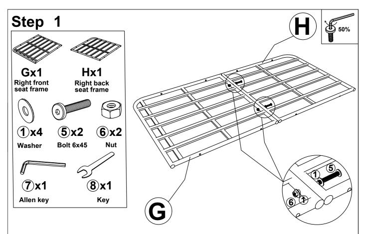
Connect The Right front seat frame (G) & Right back seat frame (H), tighten Bolt (5), Nut (6), Flat Washer (1) With Allen key (7), Key (8)
