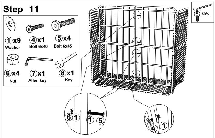
Connect The part from Step (5) & part from Step (10), tighten Bolt (4), Bolt (5), Nut (6), Flat Washer (1) With Allen key (7), Key (8)
