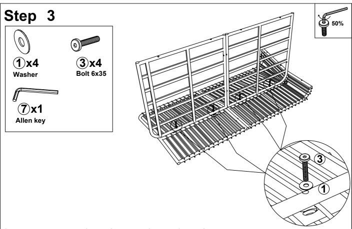
Connect The part from Step (1) & part from Step (2), tighten Bolt (3), Flat Washer (1) With Allen key (7)
