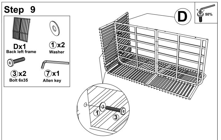
Connect The part from Step (8) & Back left frame (D), tighten Bolt (3), Flat Washer (1) With Allen key (7)
