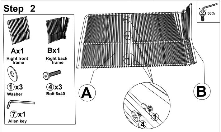
Connect The Right front frame (A) & Right back frame (B), tighten Bolt (4), Flat Washer (1) With Allen key (7)
