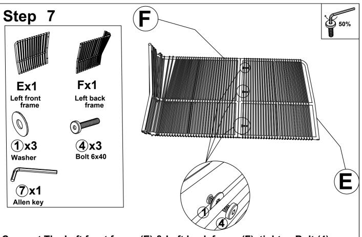
Connect The Left front frame (E) & Left back frame (F), tighten Bolt (4), Flat Washer (1) With Allen key (7)
