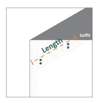
(3). Drill holes in roof with 0.19" (4.8mm), diameter drill bit, depth **1.57**" (40mm).
