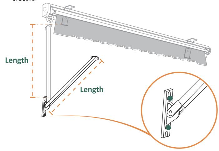
(3). Connect one end of the arm (#B) to the awning by the M6 bolt set (#F).
