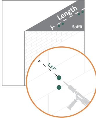
(4). Attach the wall bracket (#D) to the wall/ ceiling through expansion bolt (#E1)/ wood screw (#E2).
