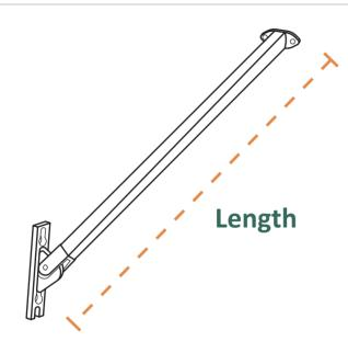
(2). Marking position: the vertical distance from the awning to the arm installation position is the length of the arm.
