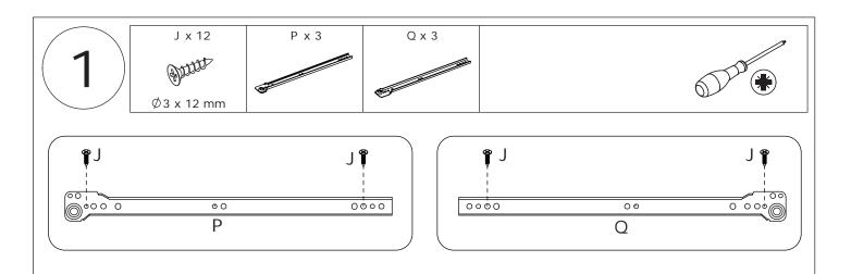
Fix slide rail(P) and (Q) to panel 5 and 6 with screw(J) at first.
