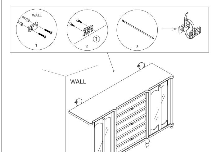
Install anti-tipping device as shown.
