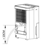
Make sure the connection between pipe and the drain outlet is tight and does not leak. Then direct the pipe to a suitable drainage poit. This unit uses gravity to dispose of water, hence the drain should be lower than the water outlet on the unit. Be sure to run the water, hence the water pipe downward and let the water to flow out smoothly. Do not kink or bend the pipe.
