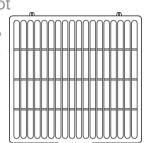
Remove the filter frame. If the optional activated carbon filter is fitted, remove them from the frame and hoover gently approximately every 2-3 weeks.
