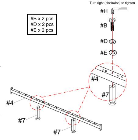
Adjust the levelers on the support rail legs (#7) according to the ground level on Step 4.
