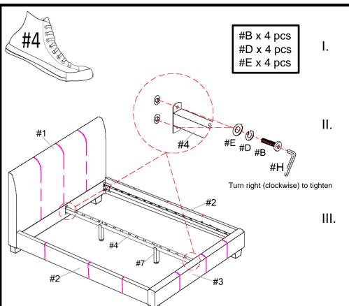
Align the assembled support rail (#4) with the pre-drilled holes on the center of the headboard (#1) and the footboard (#3). Prepare 4 bolt assemblies by inserting FIRST the lock washer (#D) onto the bolt (#B) and then the flat washer (#E) onto the SAME bolt (#B), in that order. Insert the bolt assemblies through the brackets of the support rail (#4) using the Allen wrench (#H) to lock them with the headboard (#1) and the footboard (#3).
