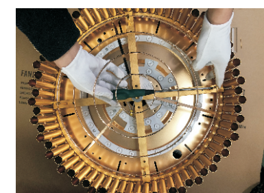
Step 7. Install the lamp shade round crystal lifting ring on the corresponding screw hole and tighten it with a tool.
