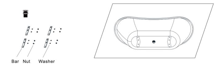
2. Assemble the drainer as below diagram, put this part ① on the drainer hole, put this part ② under the drainer hole, must be tighten up to prevent water leakage.
