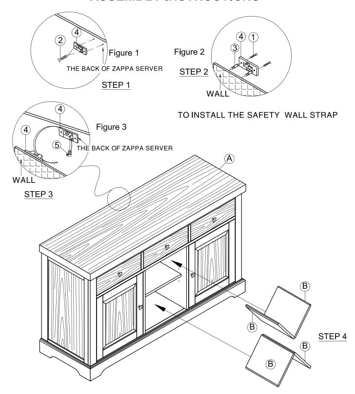
Step 1: To prevent the Zappa Server from tipping, follow the instruction shown here: Put the Mounting Plate (4) to the backside of the Zappa Server, using 2 Short Screw (2) to secure in place. See Figure 1.
