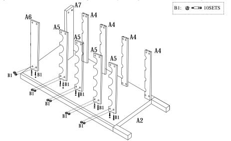
Step 5: Assemble the side panel A3 to the wine racks A4,A5 and back panel A6 and the front panel A7 using camlocks B1 as below drawring shown.
