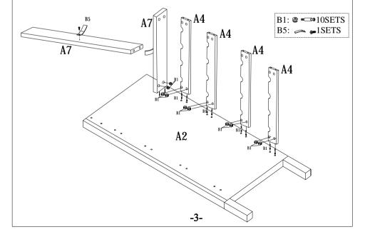
Step 3: Assemble the back panel A6 to the side panel A2 useing camlock B1 as below drawing shown.
