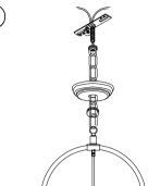
5. Open the quick link at one end of the CHAIN, attach it to the HANG STRAIGHT, let the cable go through the CHAIN. 6. Release the FASTENER RING from the HANG RING.let the **FASTENER RING and CANOPY**
