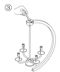
3.Attach one end of the WOOD FRAME to the CYLINDER UP, fastenit by the screw nuts.
