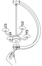
4. Attach the other end of the WOOD FRAME to the CYLINDER DOWN, fasten it by the screw nuts.
