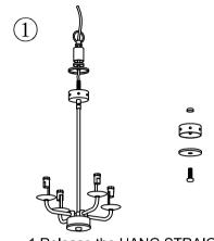
1.Release the HANG STRAIGHT and FASTENER from the CYLINDER UP and DOWN,take out the CYLINDER COVERS. Fasten the ROD to the rod joint of the lamp body.
