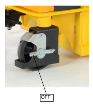
To release the parking brake, press down on the brake pedal
