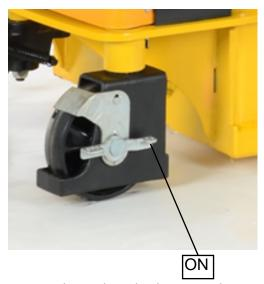
To activate the parking brake, press down on the brake pedal
