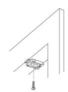
When turning the screw, do not over tighten. Overtightening can put pressure on the inner bracket and constrict movement, preventing the inner part of the bracket from latching to the headrail. If you find the headrail will not latch to the bracket, try slightly loosening the screw.
