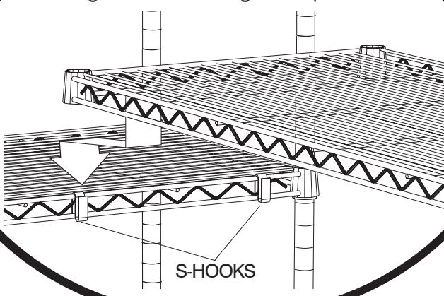
**7** Snap half-sleeve sets onto add-on posts at same height as next shelf on starter unit. Lower the next shelf into position with the shelf frame of the non-post side on the S-hooks. Press corners near half-sleeves until fully seated. Install the third and fourth shelves in the same manner.
