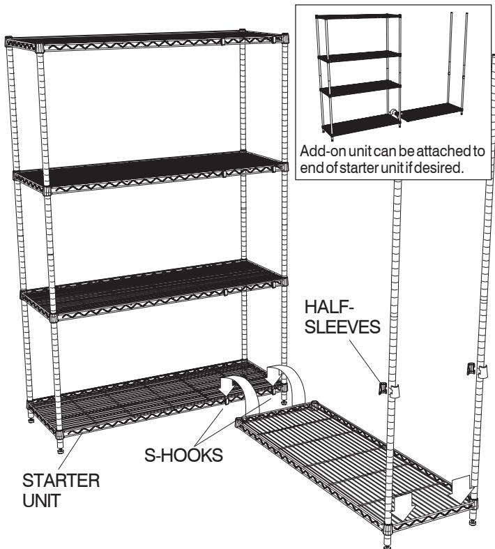
Connect add-on shelf to corresponding shelf on main unit using two S-Connecting Hooks per shelf.
