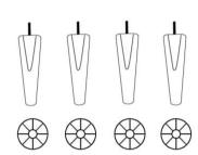
2. Screw in the feet (B) into the screw holes underneath the base using the plastic washers (C)
