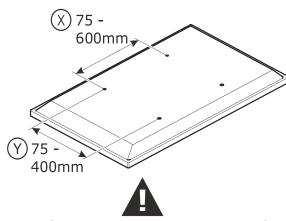
If width  $\bigotimes$  is greater than 600mm or height  $\bigotimes$  greater than 400mm STOP installation now and contact the customer help line
