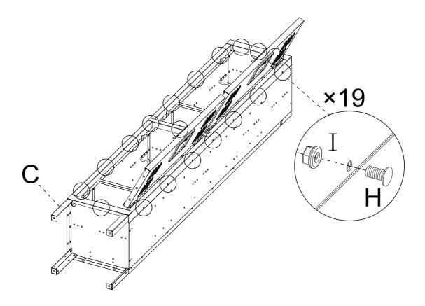
Snap on the door panel and install the nuts from the inside.
