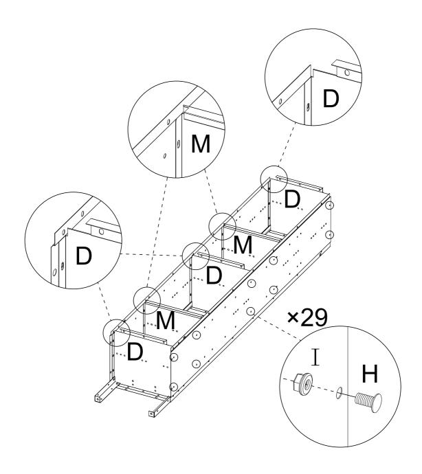
Assemble 3 Parts D, 2 Parts M, back plate B and side plate A with H\*29 bolts and I\*29 nuts (Install the hook installed part D on the upper part of the cabinet)
