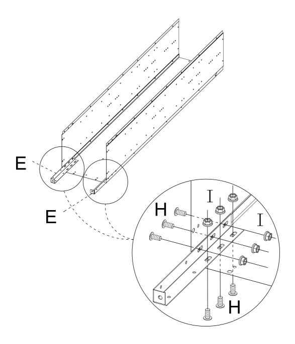
Attach the two legs, using six bolts and nuts to secure each leg, taking care to push the leg to the top of the hole to keep it aligned with the front leg.
