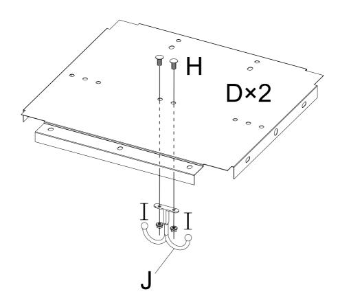
Fix hook J\*2 to parts D with bolts H\*4 and I\*4 nuts(Fix hooks on two parts D only)
