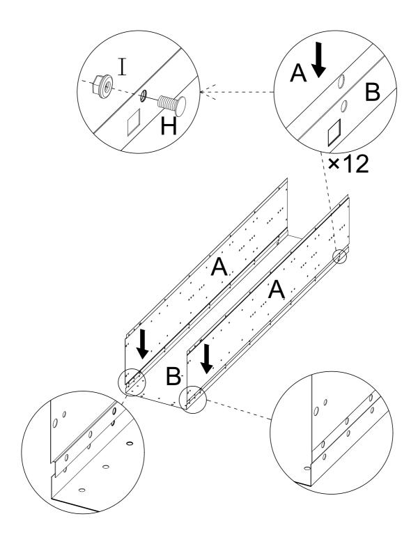
Overlap the two side walls with the vertical part of the back wall and secure them with six bolts and nuts on each side.
