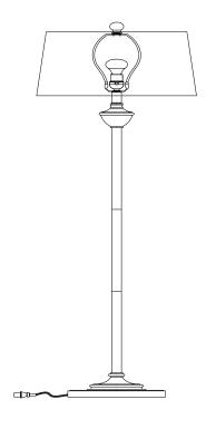
Step 1 Make sure all parts could be aligned before assemble Do not rotate lamp body too hard avoid base screw broke Put the shade(F) on the Harp(E), then Screw the Lamp body (B) onto the Lamp base (A)
