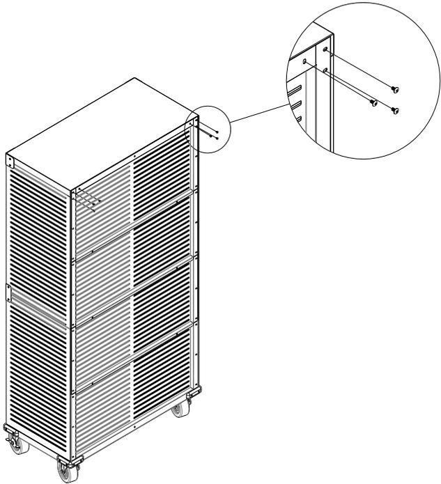
**Step 10: Remove the 6 corner screws from the top back panel of 16236.**
