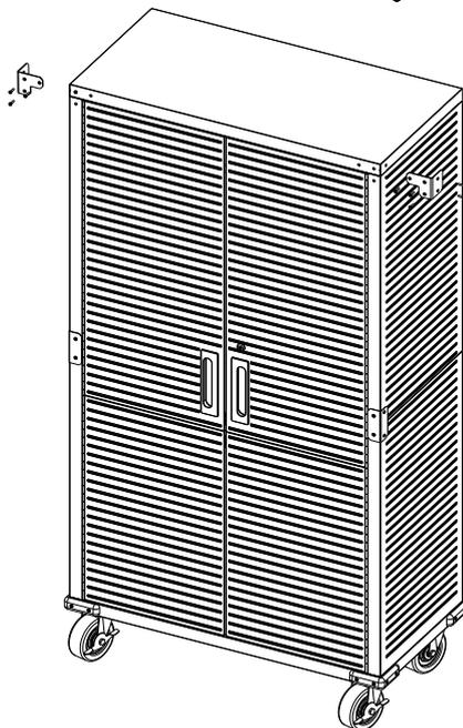
**Step 9: Remove the top Corner Protection brackets from Model No. 16236 /20143B Tall Cabinet as the left photo shows.**
