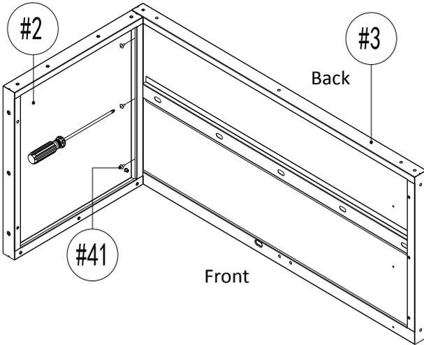
**TIP: A magnetic screwdriver is included for your convenience. If a power screwdriver is used, keep on a low torque setting.**
