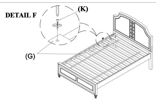
6. Place Slat roll (G) to the Side Rails (F). Screw in (K) on each end of the Slats Frame. As shown in **DETAIL F**.
