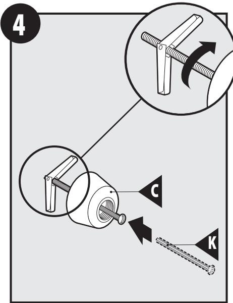
1. Insert Bracket Screw (K) into front end of opening of Escutcheon (C).
