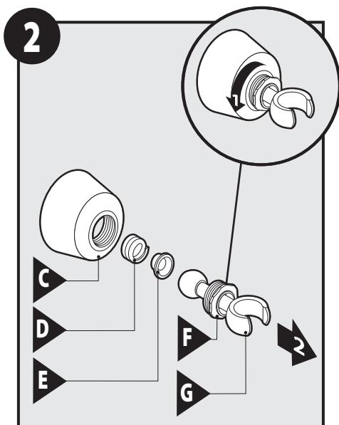
1. Loosen Wall Bracket Nut (**F**) from Escutcheon (**C**).
