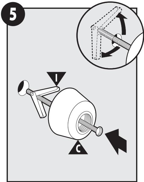
1. Install Bracket Toggle (I), Bracket Screw and Escutcheon (C) into shower wall opening. Pinch ends of toggle bracket to fit into hole.
