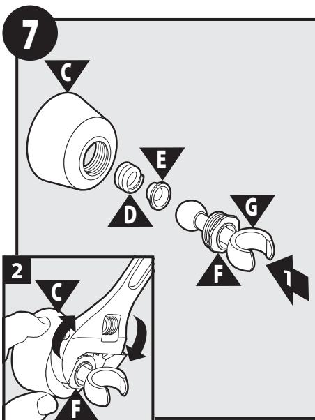
1. Re-install Spring Coil (D), Washer (E), Wall Bracket Nut (F), and Wall Bracket Hook (G) back into Escutcheon (C).
