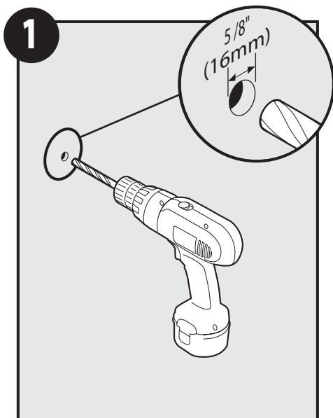
Drill 5/8" hole in shower wall with 5/8" drill bit.
