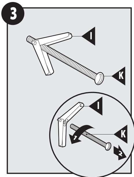
1. Unthread Bracket Screw (K) from Bracket Toggle (I).
