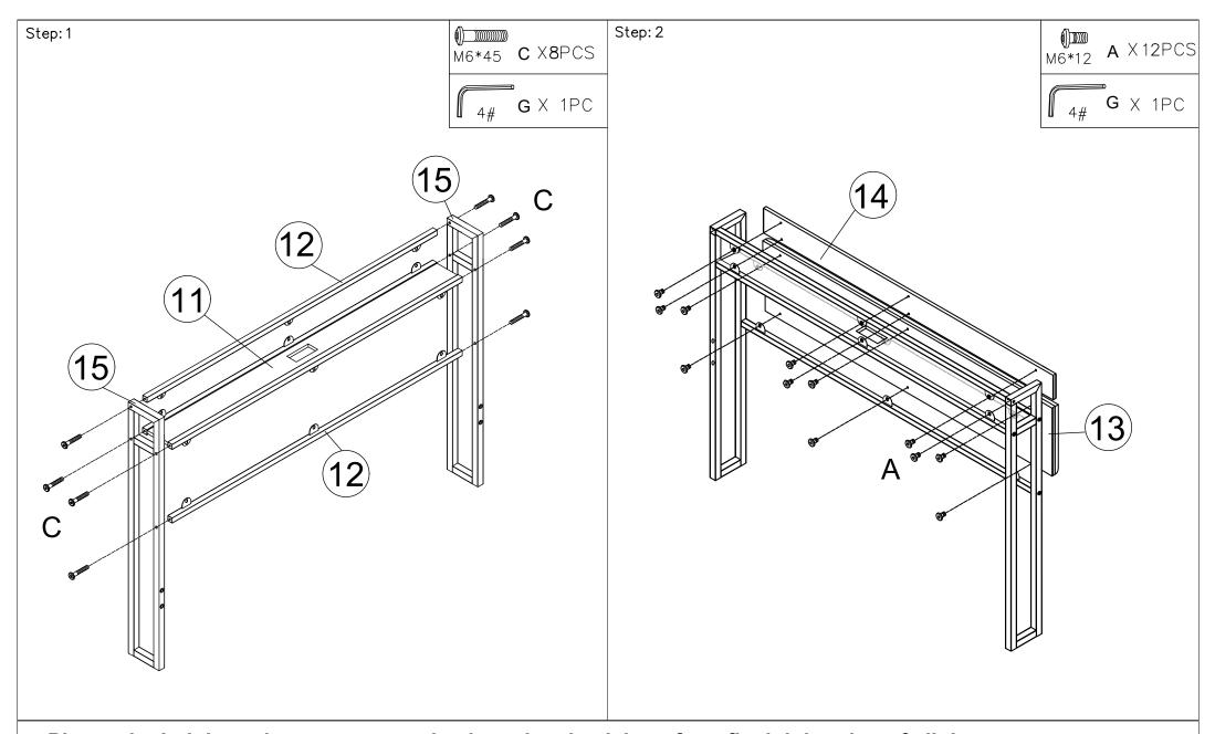
Please don't tighten the screws completely and go back later for a final tightening of all the screws after pieces are aligned with each other.
