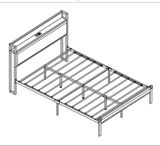
Attention: Please don't tighten the screws completely and go back later for a final tightening of all the screws after pieces are aligned with each other. If the screws are tightened initially, subsequent hole positions may be misaligned.
