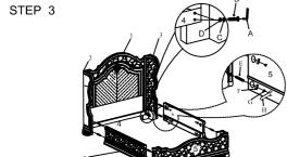
Fasten the bolts after alignment for the bottom line of FB to rails
