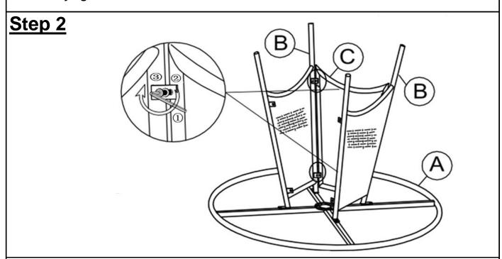
Attach Leg Support Panel(C) between Leg Panels(B) using Bolt(3) and Washer(2) with Allen Key(1) as shown in the picture above.
