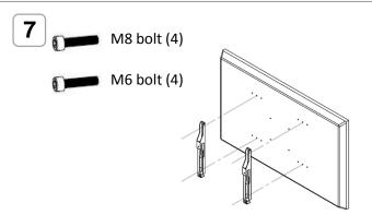
Before installing mounting brackets attach these to TV and secure tightly before mounting.
