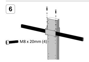
Insert (2) M8 x 20mm bolts on the top and bottom of tube bracket to secure it. Use the hex key to tighten.
