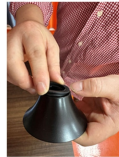
Step 6. Put the horn cover in the rubber ring
