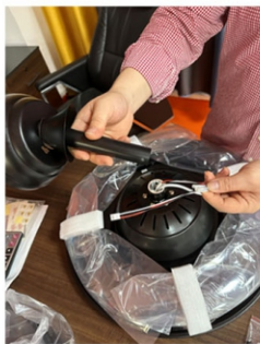
Step 8. Run all the wires through the boom
