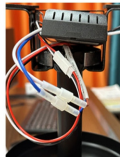
Step 16. Place the connector in the mounting bracket to secure it
