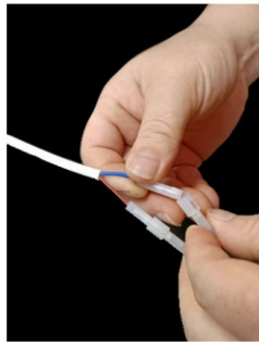
Step 2. Blue to blue line, brown to brown line insert connection
