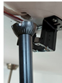
Step 12. Install the support Place the boom with the sling in the mounting support
