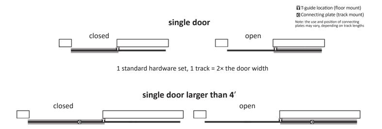
1 standard hardware set, 2 or 3 tracks = 2× the door width, connecting plate(s), extra wall mount kit(s)
