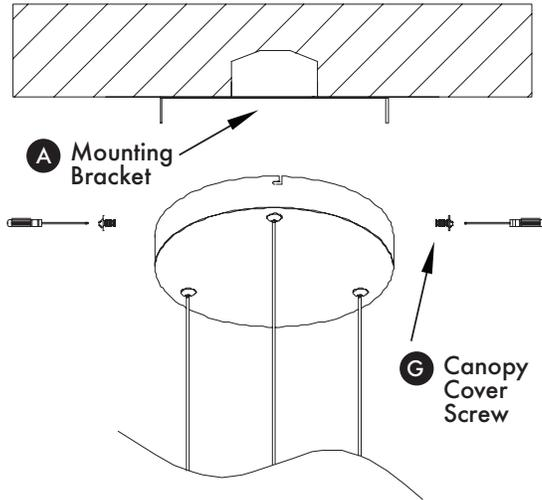
Secure canopy to mounting bracket (A) with canopy cover screws (G).
