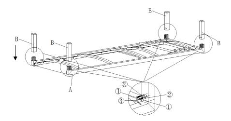
Open the carton and place all the parts onto a clean, non-marring surface. Place the Seat Panel(A) facedown.
