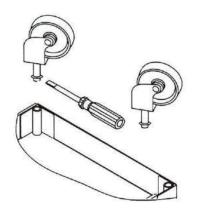
Insert the wheels into the bottom holes of the cabinet.
