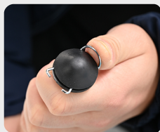
Press the wheel cap wire and install it onto the wheel rod
