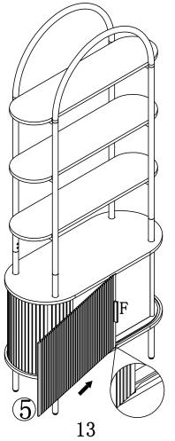
Board 5 should be aligned with the upper and lower slots before being pushed out
